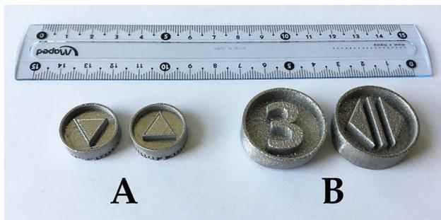
**Fig. 9** (A) 20 mm diameter (5 mm bulk metal (Ti6Al4V here, but possible CuNi2SiCr) at the bottom and 5 mm dented for filling with ceramic (TiO<sub>2</sub>-Cu or TiO<sub>2</sub>-Ag in SPS process), and (B) 30 mm height (10 mm bulk metal at the bottom and 10 mm dented for filling with ceramic in SPS process) applied for elevator buttons
