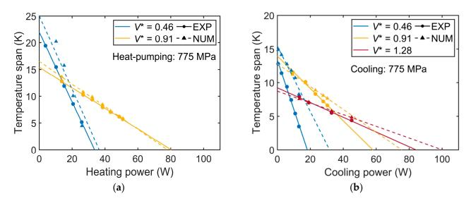
**Figure 8.** Comparison between experimentally determined and numerically calculated temperature span—cooling/heating power characteristics for heat-pumping (**a**) and cooling (**b**) at a stress level of 775 MPa.
