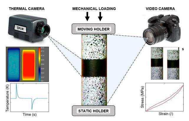
**Figure 1.** Schematic representation of the experimental setup for superelastic and elastocaloric characterization of the tube, showing the tube with the marked regions of interest for the thermal camera and video extensometer measurements.
