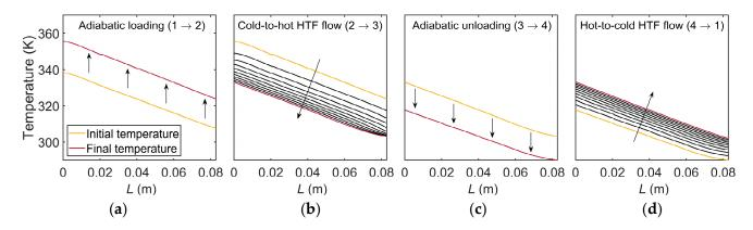
**Figure 6.** Evolution of the eCM temperature profile along the AeCR during each phase of the thermodynamic cycle.
