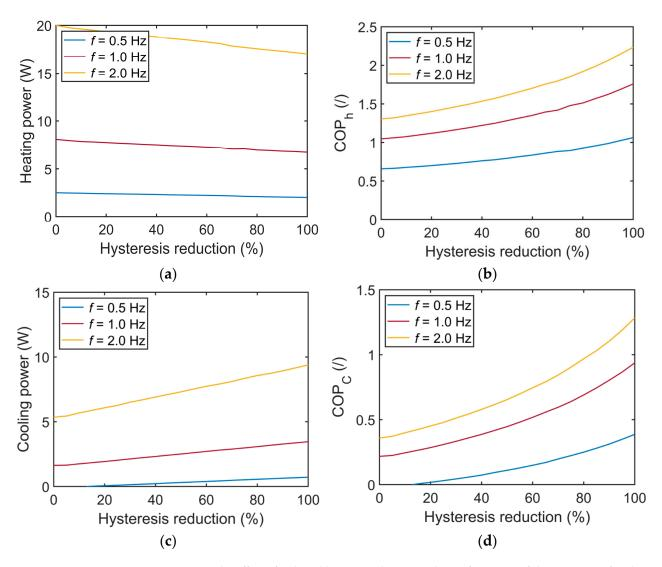
**Figure 13.** The effect of reduced hysteresis losses on the performance of the AeCR at a fixed strain of 2.7%, temperature span of 15 K and displaced fluid volume ratio of 0.6 for heat-pumping (**a**,**b**) and cooling (**c**,**d**).
