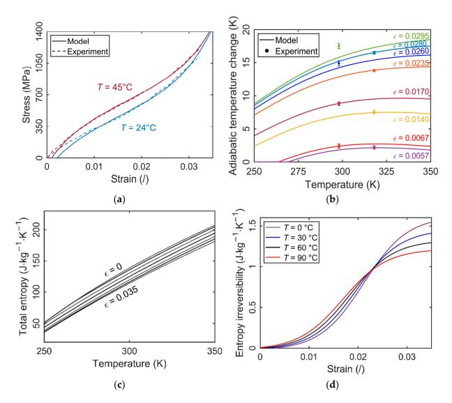
**Figure 3.** Comparison of experimentally determined and modeled superelastic behavior at different temperatures (**a**); comparison of experimentally determined and modeled positive adiabatic temperature changes during loading (**b**); entropy-temperature diagram (**c**); Modelled entropy irreversibilities as a function of strain at different temperatures (**d**).
