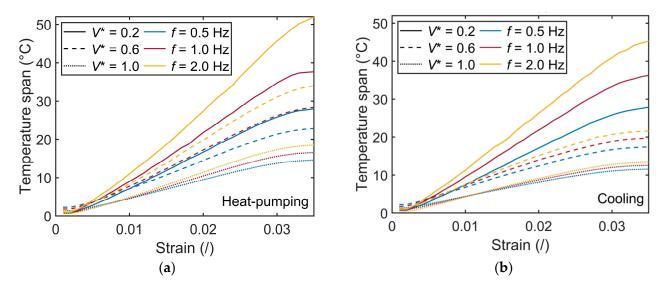
**Figure 10.** The effect of different applied strains at different operating conditions (operating frequency and displaced fluid volume ratio) on established temperature spans at no thermal load conditions for heat-pumping (a) and cooling (b).
