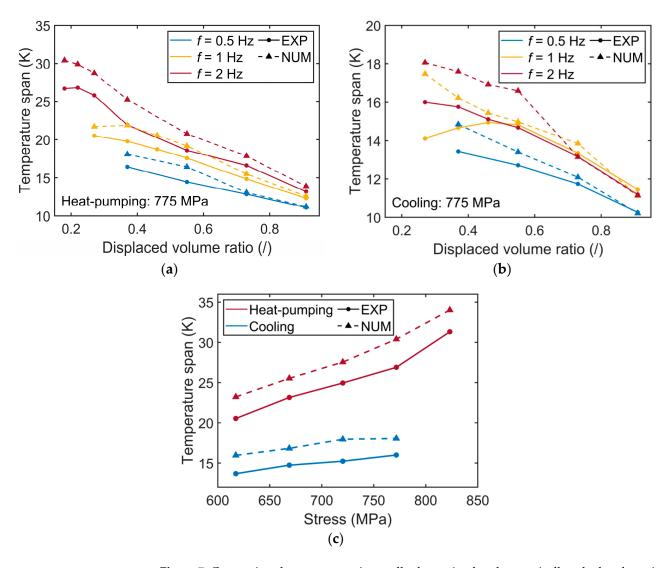
**Figure 7.** Comparison between experimentally determined and numerically calculated maximum temperature spans established along the AeCR under different operating conditions for heat-pumping (a) at a stress level of 775 MPa and cooling (b) and under different mechanical loads (c).
