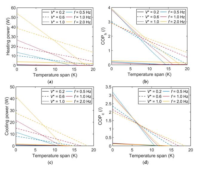
**Figure 11.** The effect of temperature span on AeCR performance at a fixed strain of 2.7% for heat-pumping (a,b) and cooling (c,d).
