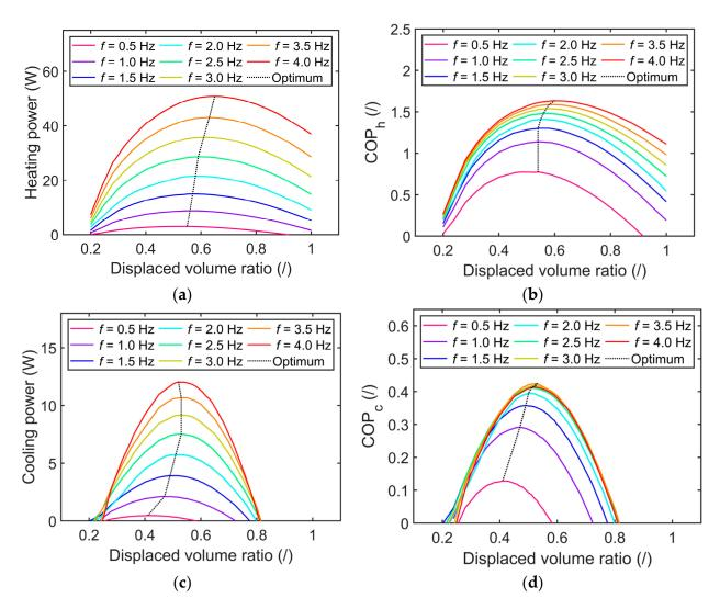
**Figure 12.** The effect of displaced volume ratio and frequency on AeCR performance at a fixed strain of 2.7% and temperature span of 15 K (based on inlet fluid temperatures) for heat-pumping (**a**,**b**) and cooling (**c**,**d**).
