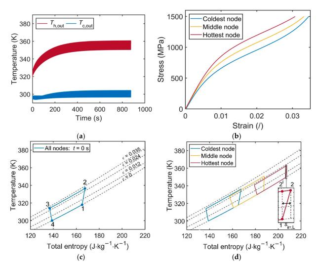
**Figure 5.** Time evolution of the temperature span of HTF outlet temperatures (a); presentation of the modeled loading curves at three different temperatures (b); presentation of the modeled active elastocaloric cycle in the T-s diagram with detail of the inclusion of irreversibility in the case of the first cycle (c) and the steady-state cycle (d).
