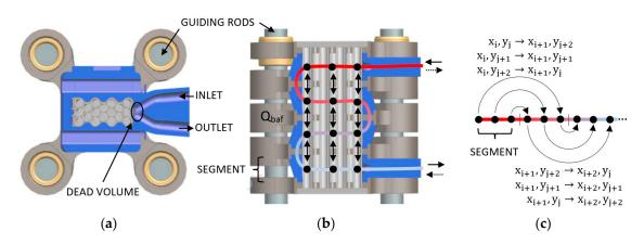
**Figure 4.** CAD model of the shell-and-tube AeCR: cross-sectional view (a); longitudinal view with a schematic representation of the 1D discretization of regenerators' domain (b); and schematic representation of the heat transfer through the baffles in the 1D domain (c).
