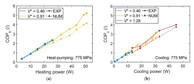
**Figure 9.** Comparison between experimentally determined and numerically calculated COP—cooling/heating power characteristics for heat-pumping (a) and cooling (b) at the stress level of 775 MPa.
