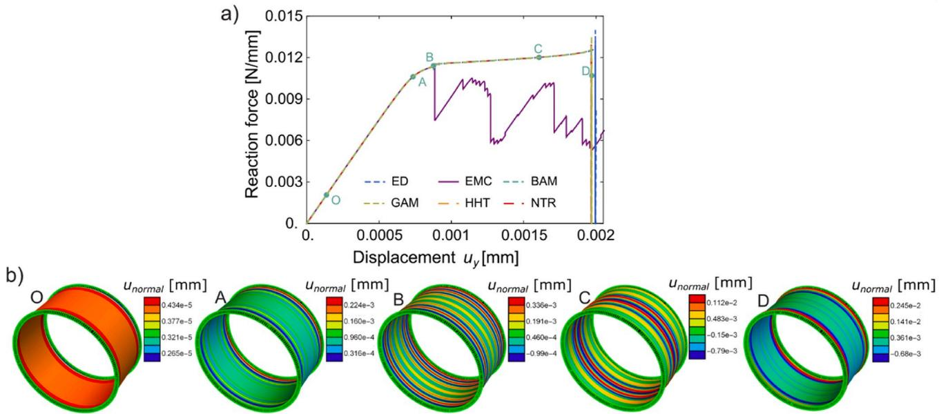
Fig. 10. Configuration CS4. a) Force-displacement response. b) Deformed shell configurations at various points on the above diagrams.
