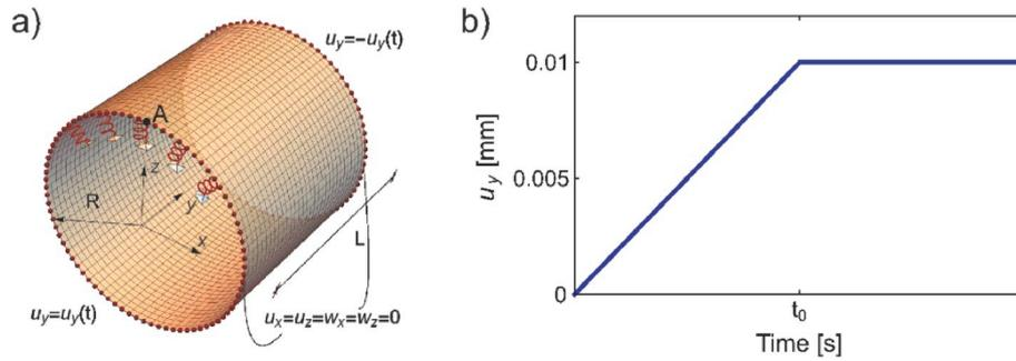
**Fig. 3.** a) Finite element model (the springs are distributed across the entire inner surface). b) Loading function.
