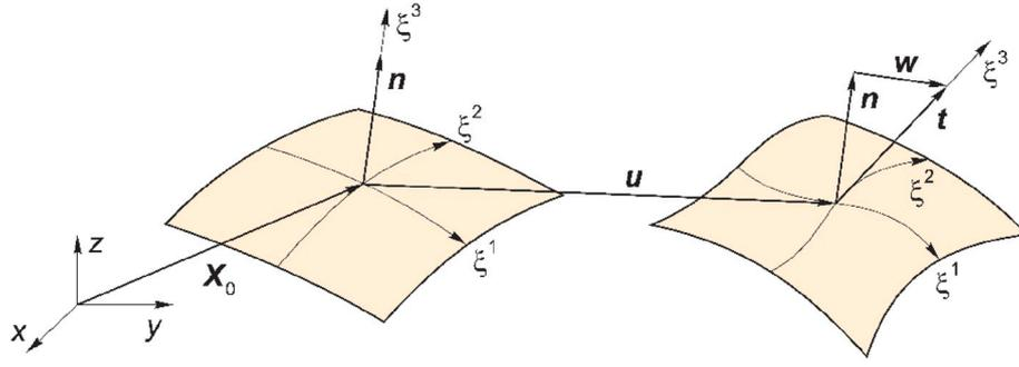
Fig. 1. Shell model kinematics.
