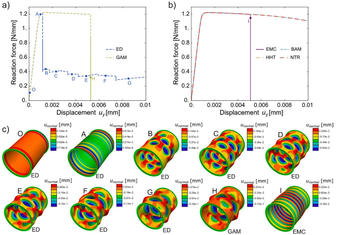
**Fig. 8.** System CS3. a) Force-displacement response for ED and GAM. b) Force-displacement response for EMC, BAM, HHT and NTR. c) Deformed shell configurations at various points on the above diagrams.
