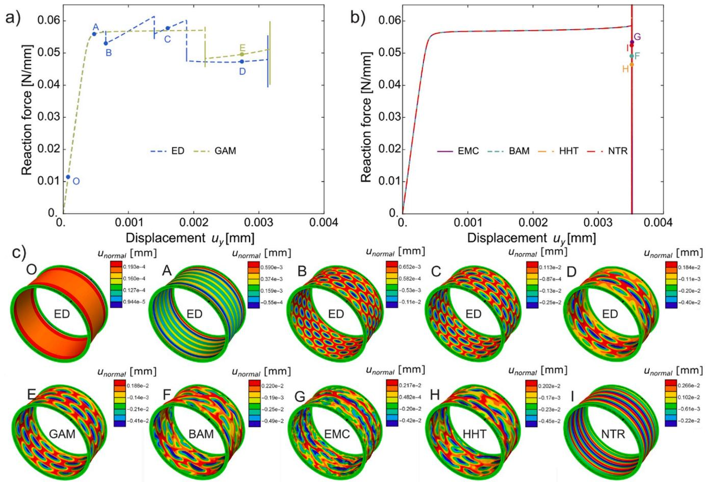
**Fig. 4.** System CS1. a) Force-displacement response for ED and GAM. b) Force-displacement response for EMC, BAM, HHT and NTR. c) Deformed shell configurations at various points on the above diagrams. Patterns in configurations F–I are oscillating due to the un-damped vibrations.
