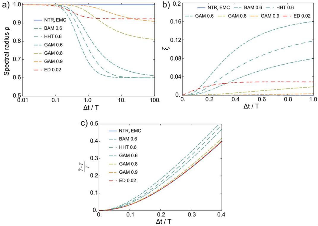
Fig. 2. Properties of used time integration schemes. a) Spectral radius, b) Damping coefficient and c) Period elongation versus  $\Delta t/T$ .
