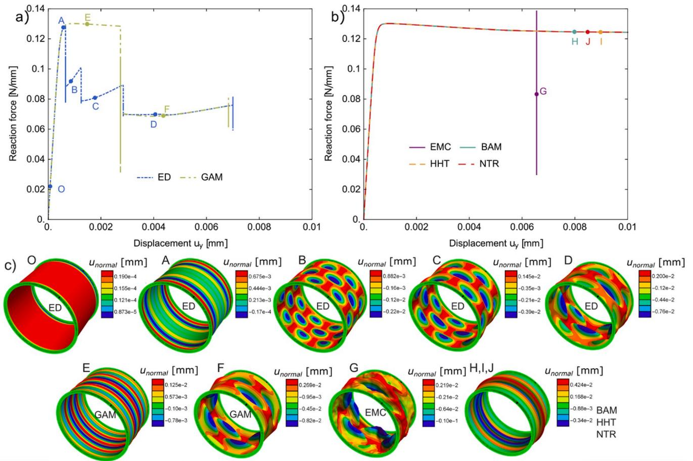
Fig. 6. System CS2. a) Force-displacement response for ED and GAM. b) Force-displacement response for EMC, BAM, HHT and NTR. c) Deformed shell configurations at various points on the above diagrams. Pattern in configuration G is oscillating due to the un-damped vibrations.
