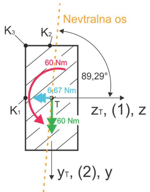
$$\sigma_{P,K_1} = \sqrt{\sigma_{K_1}^2 + 3\tau_{K_1}^2} = \sqrt{(-90,16 \text{ MPa})^2 + 3 \cdot (55,82 \text{ MPa})^2} = 132,2 \text{ MPa}$$
