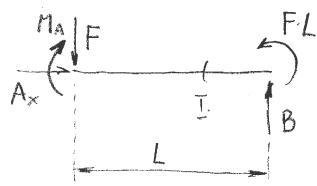
$$\begin{aligned} A_x &= 0 \\ B - F &= 0 \\ FL + FL - M_A &= 0 \\ B &= F \\ M_A &= 2FL \end{aligned}$$
