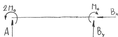
$$\begin{array}{l} M \\ \left( \begin{array}{c} M_0 \\ M_0 \\ \frac{M_0}{L} \end{array} \right) \end{array} \quad M + M_0 + \frac{M_0}{L}x = 0 \\ M = -M_0 - \frac{M_0}{L}x$$
