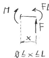
$$\begin{aligned} M - Fx - FL &= 0 \\ M &= F(L+x) \end{aligned}$$
